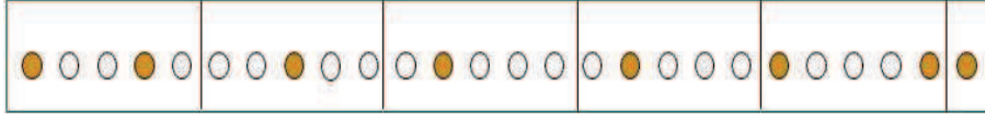
Figure 2. Piecewise random sub-sampling: the solid circle (yellow one) represents receivers, the hollow circle (white one) means no receivers. Large gap are controlled for any sampling points.
